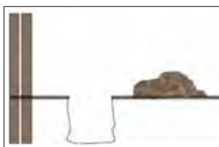
3. Dig a hole minimum 500mm deep x minimum 400mm diameter.
