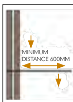
2. Soakaway should be at least 600mm from the wall to avoid causing damp to the footings.
