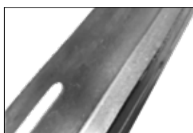
PROCESS ONE Corrosion resistant raw material, often referred to as Zintec
