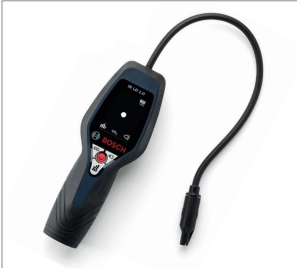
The BOSCH IR LD 1.0 CO<sub>2</sub> leak detector is specifically designed to detect R-744 - Carbon Dioxide (CO<sub>2</sub>). This leak detector meets / exceeds EN14624 performance standards with an ultimate sensitivity of less than 2 g/yr.
