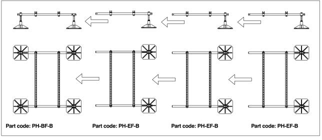
\* The system can accommodate any number of AHUs by simply adding additional PH-EF-B (extender frames)
