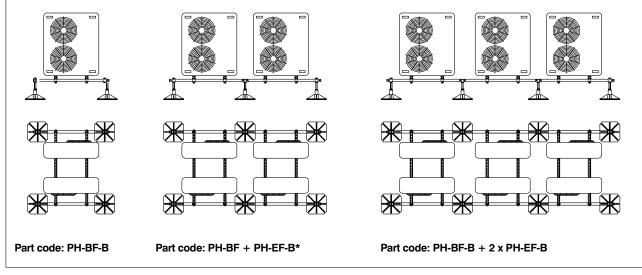
\* The system can accommodate any number of AC splits by adding additional PH-EF-B (extender frames)
